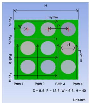
Fig. 2. Cross section of 3 by 3 rod fuel bundles and measuring location
