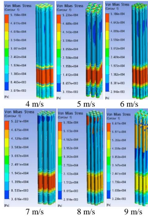
Fig. 6. Von Mises stress under different outlet flow velocity
