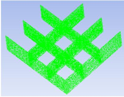
Fig. 5. Spacer grid model
