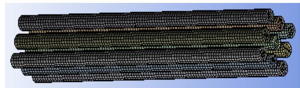
Fig. 3. Structure meshes of nuclear reactor rod
