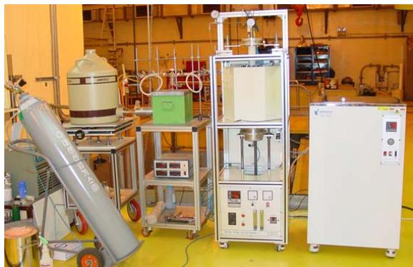
Fig. 1 The apparatus for PIA test (IMEF)
