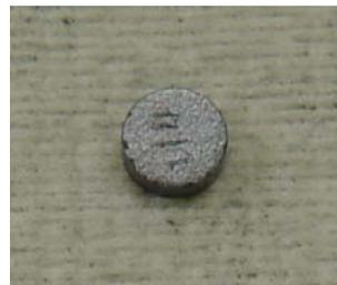
Fig. 2 UO<sub>2</sub> fuel sample
