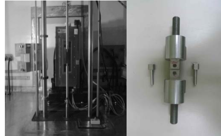
Figure 4 The UTM and the jig for fracture tests
