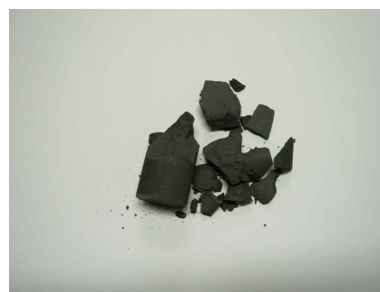
Fig. 2. Fracture shape of IG-11 graphite.
