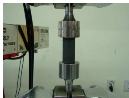
Fig. 1. The specimens of isotropic graphite IG-11 compressive test by MTS-810.
