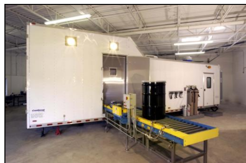
Fig. 1 Mobile Drum Venting System
