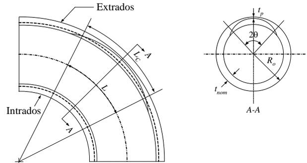
Fig. 1 Geometries of wall-thinning defect in the elbow
