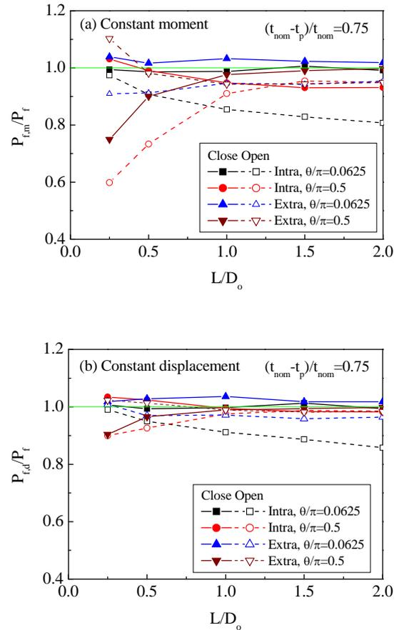
Fig. 2 Failure pressures under combined loads normalized to those under simple internal pressure
