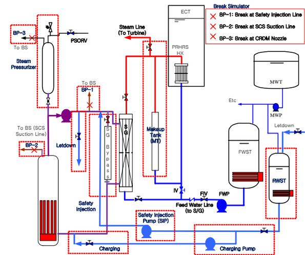
Figure 1. Schematic diagram of the VISTA ITL facility
