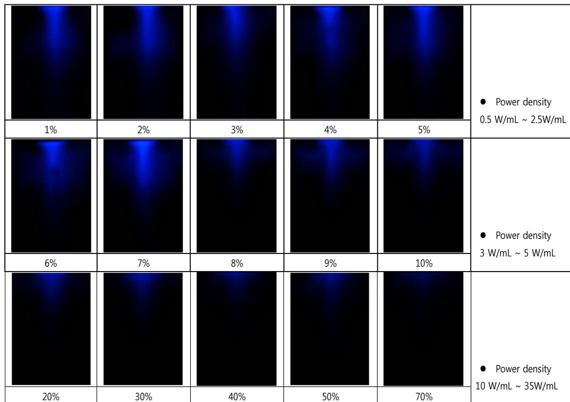
Fig. 2. An aspect of MBSL under different power density
