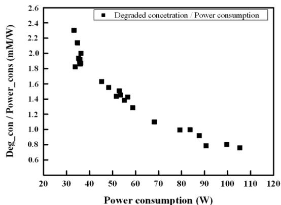
Fig. 3. At low power consumption the concentration of methylene blue was much more degraded
