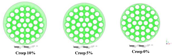
Fig 2 Positions of Bundle in Pressure Tube With Various Creep Ratios.
