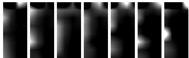
Fig. 8 visualization results of the two-phase flow measurement, 50ms interval
