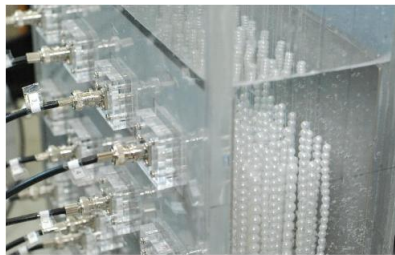
Fig. 5 Test facilities for void fraction calibration
