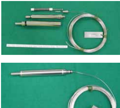
Figure 1. Parts(top) and assembly(bottom) of a dual cladding fuel rod
