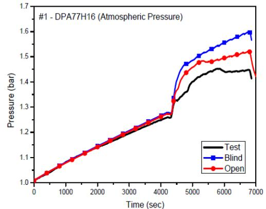
Fig. 1. Pressure buildup of HM-2 test.
