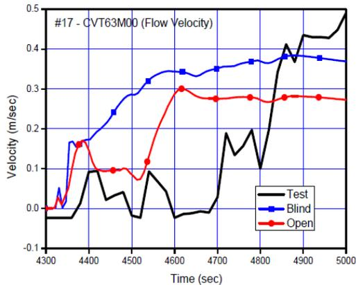
Fig. 3. Upward velocity of steam plume at the upper end of the inner cylinder at the beginning of phase 2
