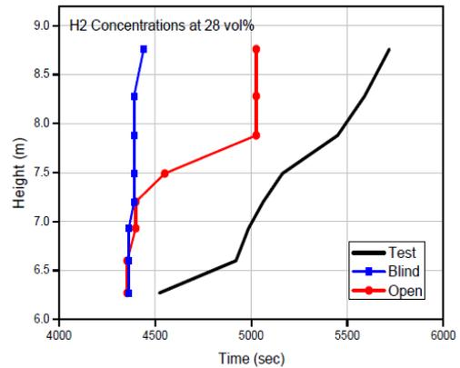
Fig. 4. Prediction of erosion process by buoyant steam against the stratified atmosphere in phase 2.
