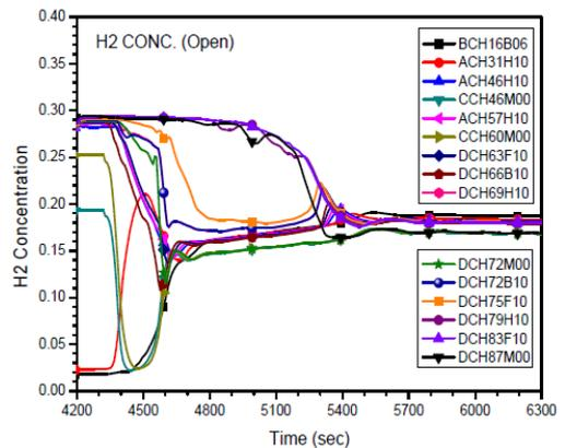
Fig. 2. Hydrogen distribution of phase 2, predicted in the open calculation. Each legend was named in accordance with the measurement in the test [2].
