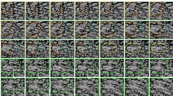
Fig. 3 Consecutive total reflection images of saturated Freon 113 pool boiling at the heat flux of 80 % CHF [time step is 1.0 ms from left to right; image size is  $4.4(\text{H}) \times 6.1(\text{V}) \text{ mm}$ ].
