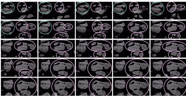
Fig. 2 Consecutive total reflection images of saturated water pool boiling at the heat flux of  $400 \text{ kW/m}^2$  [time step is 0.5 ms from left to right; image size is  $9.5(\text{H}) \times 6.1(\text{V}) \text{ mm}$ ].
