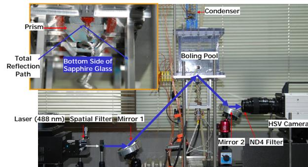
Fig. 1 Photo of the test apparatus
