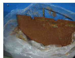
Fig. 4 Sticking of metallic oxides to cathode plate
