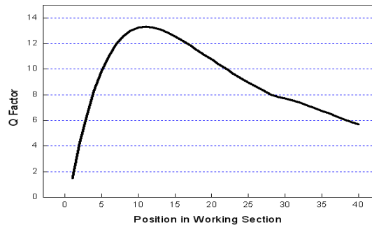
Fig. 1. Q factor values in the die working section
