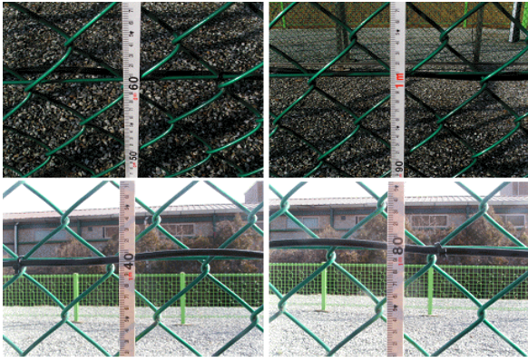
<the height of installation of the sensor line 0.6m, 1m, 1.4m, 1.8m >
