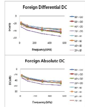
Figure 11. Depth coefficients plot of Foreign probe at differential and absolute mode
