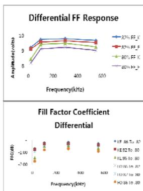
Figure 8. Fill factor coefficient comparison at differential mode
