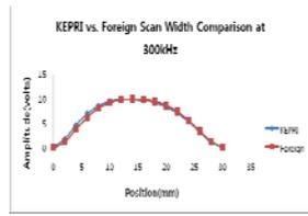
Figure 7. Scan width comparison plot for KEPRI vs. Foreign probe at 300kHz
