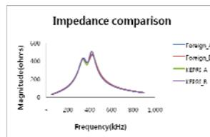
Figure 4. Impedance comparison plot for KEPRI and Foreign probe
