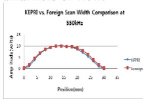
Figure 6. Scan width comparison plot for KEPRI vs. Foreign probe at 550kHz
