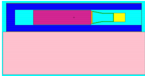
Fig. 3. A representative MCNP modeling for the spectrometer on a calibration pad (Vertical cut).
