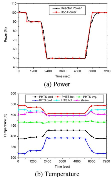
Fig. 1 Evaluation Results with constant flow rate
