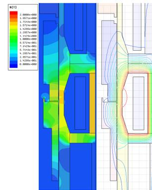
Fig. 6. Flux distribution for the case of increased turns (dr=0.25 inch)
