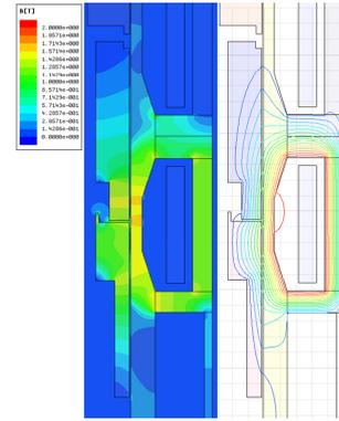
Fig. 5. Flux distribution for the case of conventional design
