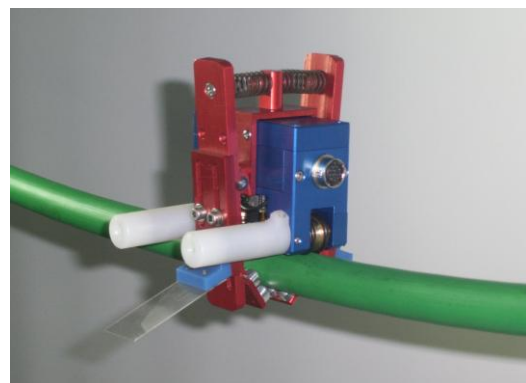
Fig. 2. Shape of the Main Robot Fixed on the Cable
