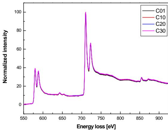
Fig. 4. Relative EELS intensity normalized with the Fe L3 edge peak maximum against the time of electron irradiation by the HVEM in KBSI
