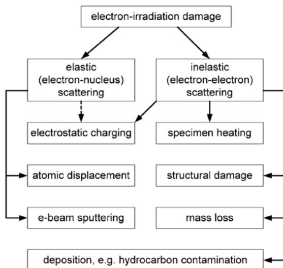
Fig. 1. Categorization of radiation damage according to the type of electron scattering and according to the effects produced in a specimen [1]
