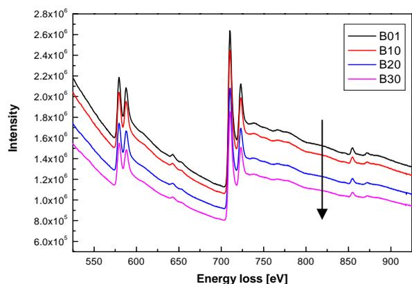
Fig. 2. EELS peaks obtained from 316 stainless steel at room temperature against the time of electron irradiation by the HVEM in KBSI.
