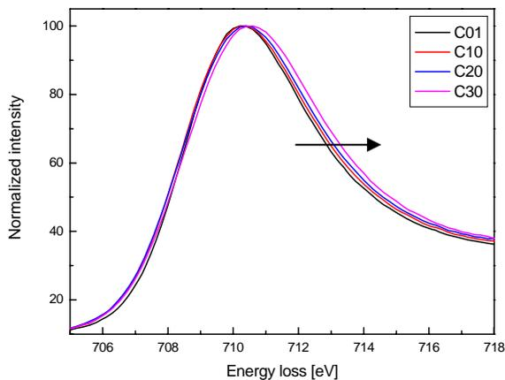
Fig. 5. Peak position and FWHM of the Fe L3 peak were increased as the time of electron irradiation increased by the HVEM in KBSI
