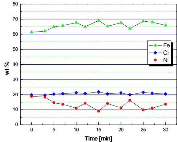
Fig. 6. Chemical composition as a function of the electron irradiation time
