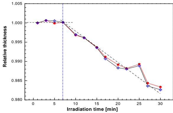
Fig. 3. The change of relative thickness versus the time of electron irradiation carried out by the HVEM.
