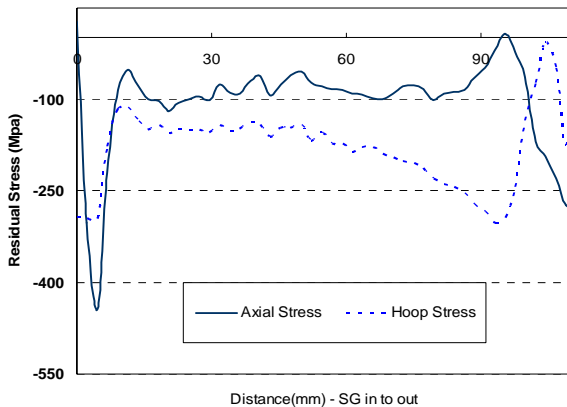
Fig. 4. Residual Stress Distribution (Roll Expansion + Weld)
