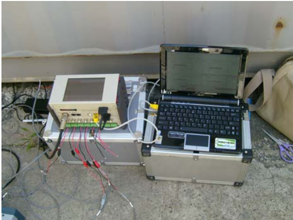
Fig. 3. The digital dynamic strain meter and the amplifier.
