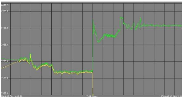
Fig. 4 Main feedwater pump speed in case of loss of one pump for 4.5% power updated Kori Unit 4.
