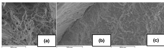
Fig.4 SEM images of fracture surfaces in the FM-52(a) at 600 °C (b) at 900 °C (c) at 1200 °C
