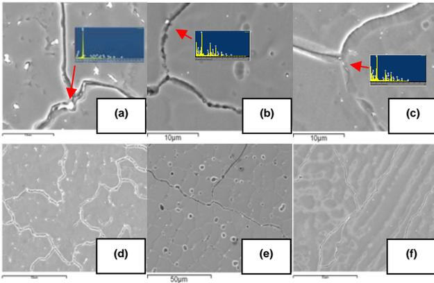
Fig.2 SEM images of FMs (a) NbCs in the FM-82 (b) TiN-like precipitates in the FM-52 (c) TiN-like precipitates in the FM-52M (d) Tortuous GBs in the FM-82 (e) Straight GBs in the FM52 (f) Straight GBs in the FM-52M.
