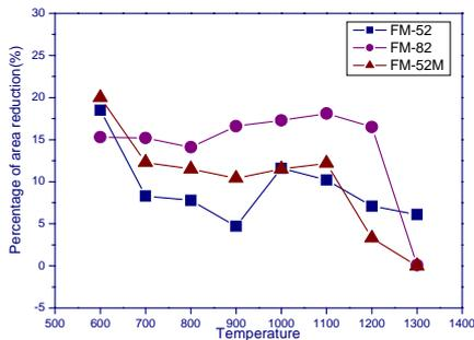
Fig.3 Hot ductility test results of FMs.
