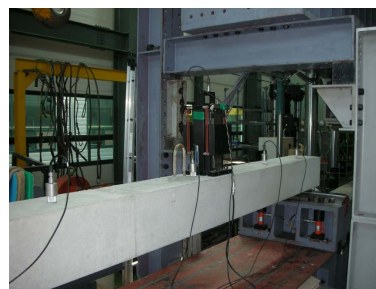
(a) Experimental modal test
