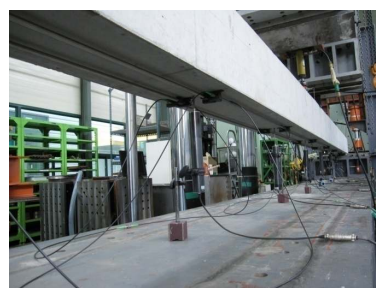
(b) Bending test by OFS and CDP
