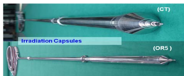
Figure 2. Irradiation capsules of CT and OR5 test holes
