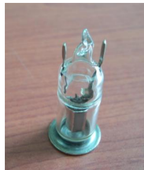
Fig. 2 Fabricated X-ray tube with a CNT fiber
