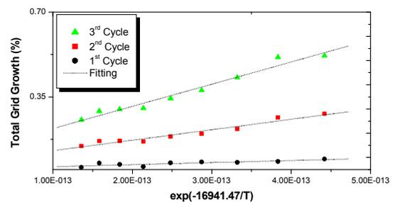
Fig.2. The measured total grid (PLUS7) growth results after each cycle of burnup in the temperature range of 570 ~ 600 °K.
