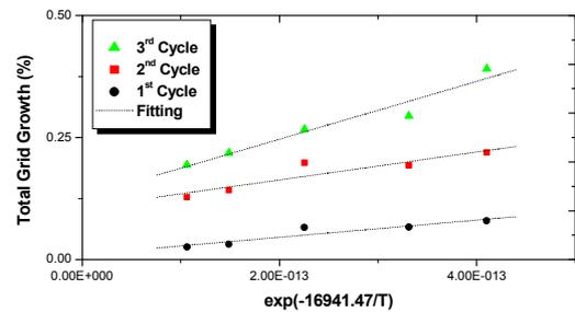
Fig.1. The measured total grid (16ACE7) growth results after each cycle of burnup in the temperature range of 560 ~ 600 °K. Total grid growth from low to high value at the same burnup represents respectively that of grid located from low to high in fuel assembly. And the linear fitting lines are shown for the further analysis of  $C_1$  constant
