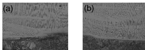
Fig. 1 Optical micrographs of as-welded specimen (a) SA508 Gr.3, (b) SA 508Gr.4N
