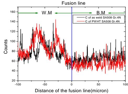
Fig. 4 EPMA data of as-welded SA508 Gr.4N and PWHT SA508 Gr.4N
