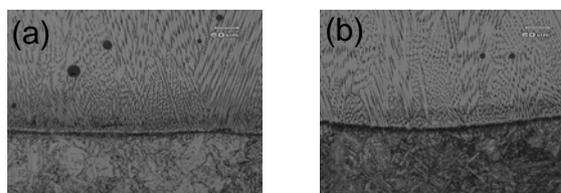
Fig. 2 Optical micrographs of PWHT specimen (a) SA508 Gr.3, (b) SA508 Gr.4N.
