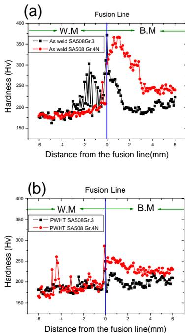
Fig. 3 The microhardness of (a) as-welded specimen and (b) PWHT specimen
