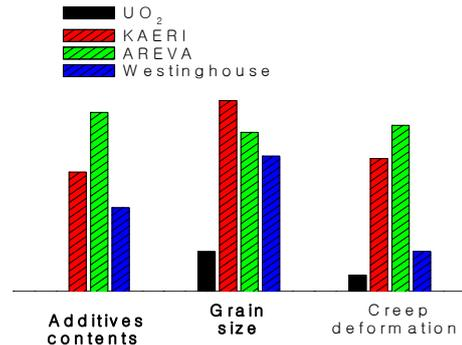
Fig. 3. Comparison of doped UO<sub>2</sub> pellets property
