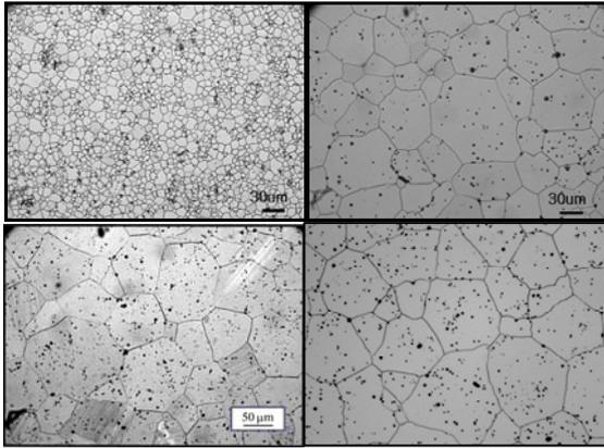
Fig. 1. Microstructure of (a) the pure UO<sub>2</sub> and (b)-(d) Mn-base additives doped UO<sub>2</sub> pellets.
