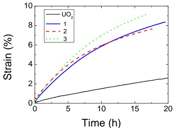
Fig. 2. Compressive creep deformation curves of the developed UO<sub>2</sub> and undoped-UO<sub>2</sub> pellets
