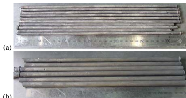
Fig. 1. Cast rods fabricated by induction melting and low pressure gravity casting; (a) U-10wt%Zr (diameter: 6 mm) (b) U-10wt%-6wt%Ce (diameter: 10 mm).
