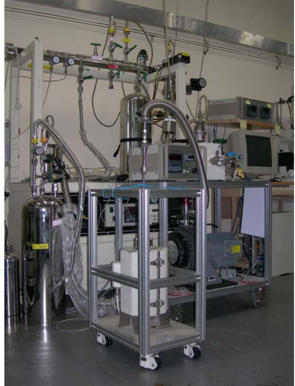
Fig.1. Hydriding/dehydriding apparatus of hydrogen.
