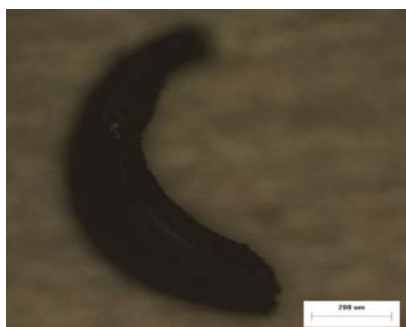
Fig.1. An O-PyC sample fragment to be measured by a density gradient column.
