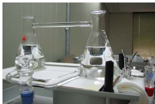
Fig.2. A flask with the lower density solution in the right side and a flask with the higher density liquid in the left side to make a density gradient solution.
