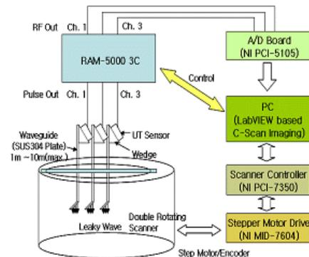
Figure 2. Experimental setup of the double rotation C-scan system
