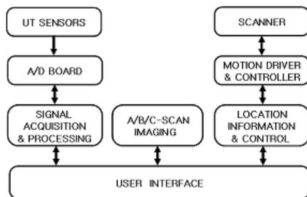
Figure 3. Data flowchart for the ultrasonic C-scan VI
