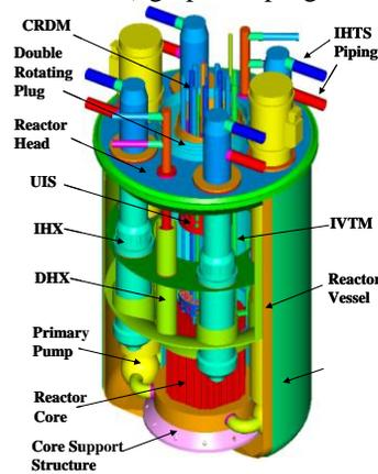
Figure 1. KALIMER-600 reactor system and double rotating plug
