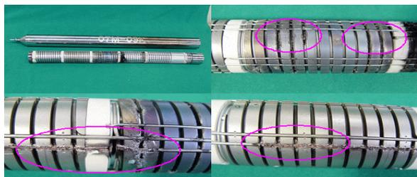
Fig 3. The damage of the heaters and thermal media
