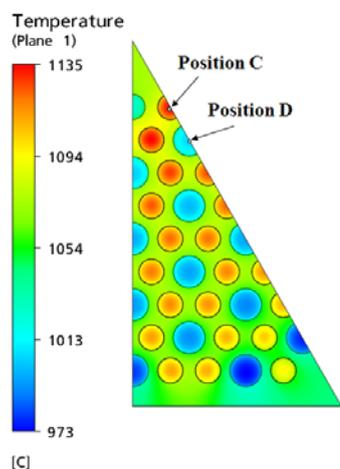
Fig. 3. Temperature contour at BOC of the hybrid shuffling core (top view at the maximum temperature plane).
