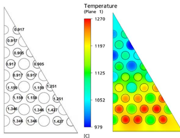
(a) Relative power within assembly (b) CFX result
