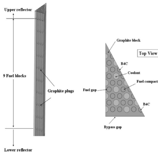
Fig. 2. Computational domain for the CFD analysis.
