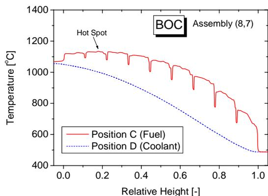
Fig. 4. Axial temperature profile of the hybrid shuffling core.
