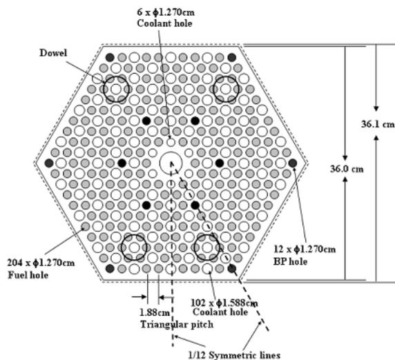
Fig. 1. The geometry of standard fuel block.
