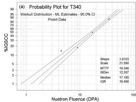
Fig. 3. The relation between %IGSCC and the neutron fluence in PWR primary water chemistry (Ref. in [4]).
