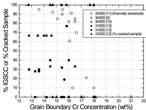
Fig. 1. Comparison between the Cr concentration at GB and %IGSCC of thermally sensitized and neutron-irradiated stainless steels in BWR normal water chemistry (Ref. in [4]).
