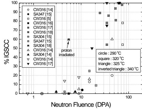
Fig. 2. %IGSCC of various stainless steels at various neutron fluence in PWR primary water chemistry (Ref. in [4]).
