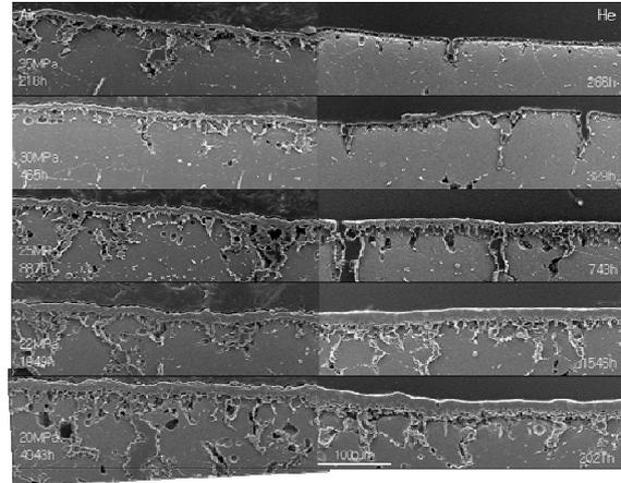
Fig. 4. Oxide layer formed on outer surface in air and He environments at 950°C
