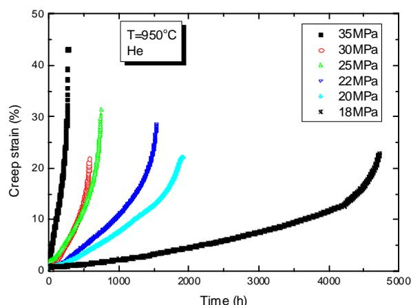
Fig. 1. Creep curves obtained with the elapsed times for different stress levels at 950°C for Alloy 617.
