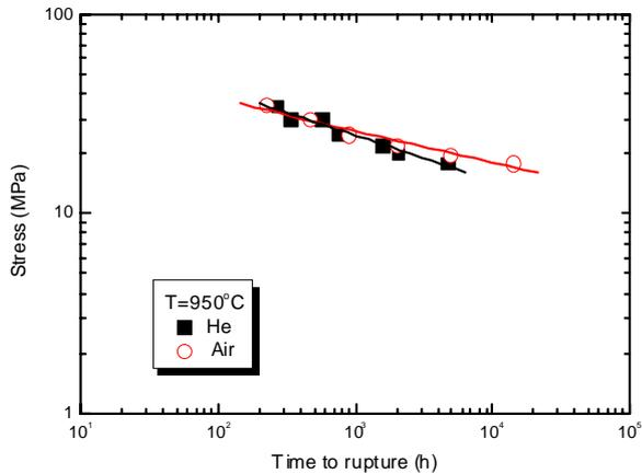
Fig. 2. Comparison of the log stress vs. log time to rupture in air and He environments at 950°C
