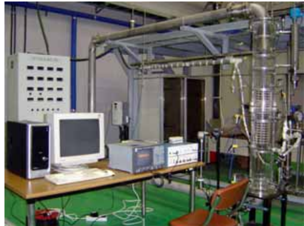
Fig. 2. The correlated active acoustic leak detection system developing in KAERI.
