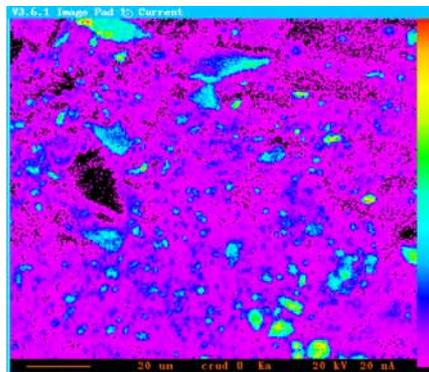
Fig.4. Image Mapping of crud deposits from the cladding interface
