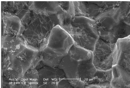
Fig.3. SEM of crud deposits from the steam generator tube plug
