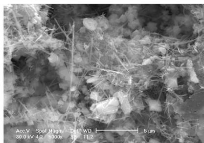
Fig.2. SEM of crud deposits from the cladding interface
