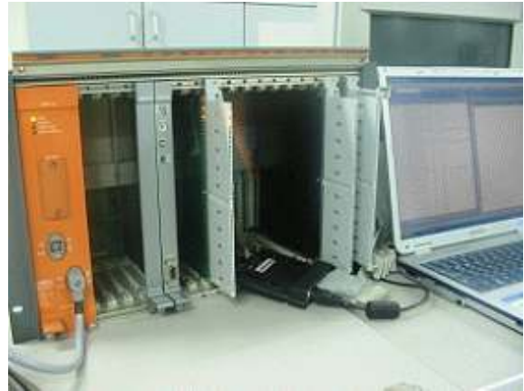
Fig. 1. Fault injection experiment environment used in the fault detection coverage estimation
