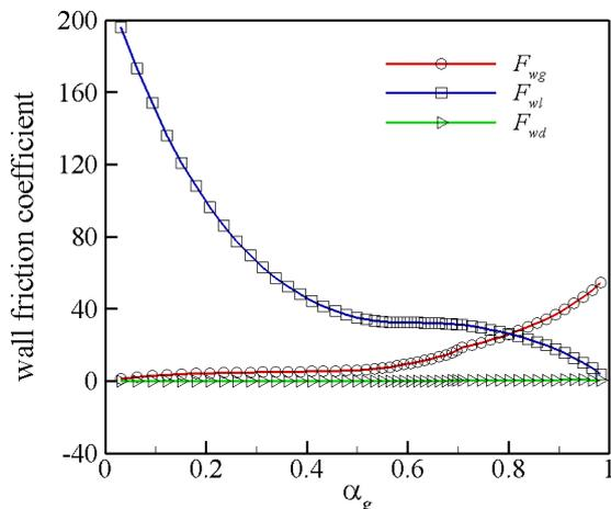
Fig. 4. Wall friction coefficient variation with void fraction
