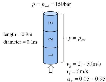
Fig. 1. Schematic diagram of a vertical test
