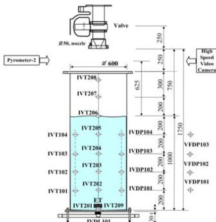
Fig. 1. Schematic diagram of the interaction vessel in the TROI facility (unit : mm).
