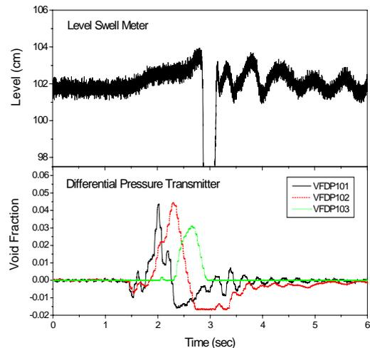
Fig. 3. Scoping test results (level swell meter and DP)
