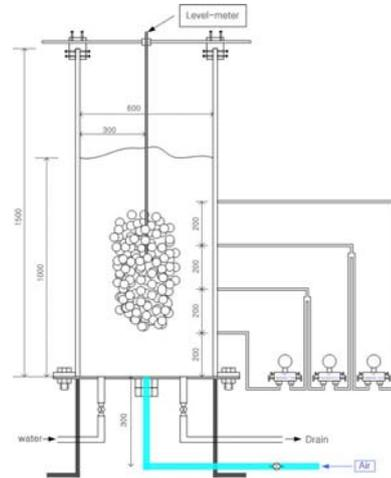
Fig. 2. Schematic diagram of the scoping test facility (unit : mm).
