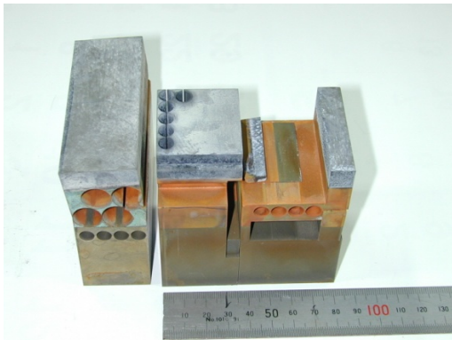
Fig. 4. Small mockup simultaneously fabricated with the qualification mockup after extracting all kinds of samples for the destructive tests.
