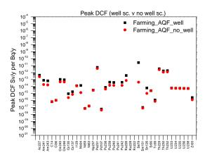
Fig.1. Peak dose conversion factors for farming exposure group due to 38 nuclides in case of Aquifer-GBI which show slight discrepancy for several nuclides by well existence.
