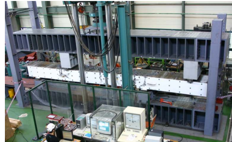
Figure 2. Loading Frame(Shear Test)
