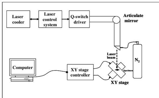
Fig.1 Schematic view of the experimental apparatus.
