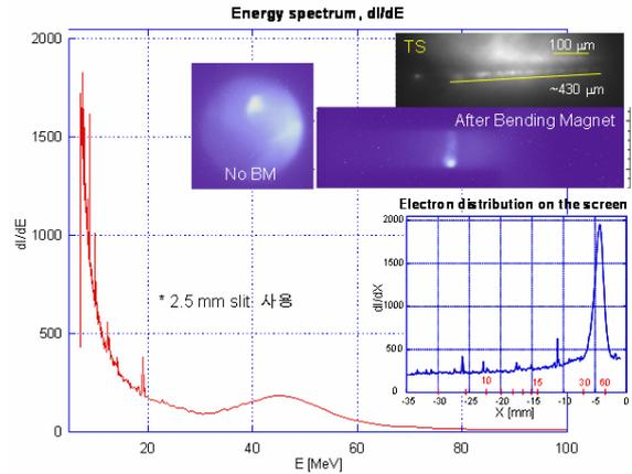
Fig. 4: Energy spectrum of laser accelerated electrons.
