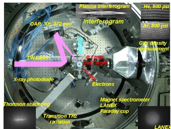
Fig. 2. Experimental set-up for Laser-induced electron generation
