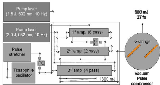
Fig. 1: Schematic of the KAERI 30 TW laser system.
