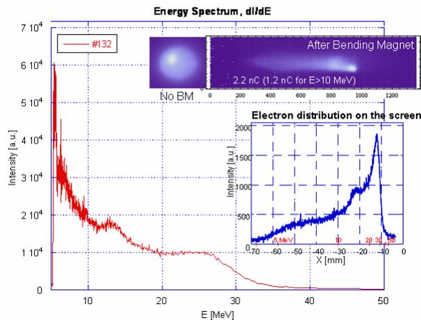
Fig. 3: Energy spectrum of laser accelerated electrons.
